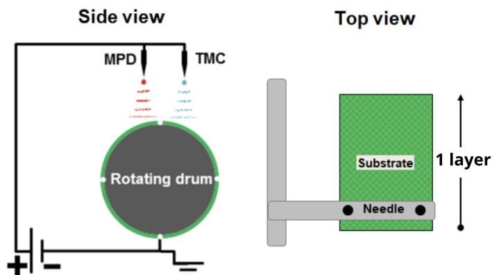
**Figure 1.** Illustration of the lab-scale electro spray process with a single drum. Monomers are deposited by a needle, sequentially, onto a substrate that is attached to the rotating drum where they react to form aromatic polyamide. The lab-scale system can make up to 1 square foot of material and is representative of a continuous process and can be expanded.
