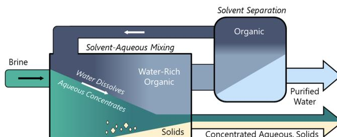
Figure 1. Conceptual design of DME-driven water selective solvent extraction.
