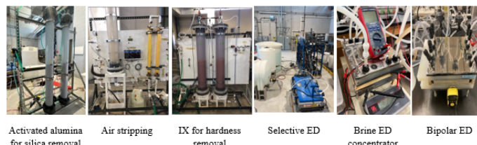
Figure 1. Overview of the pilot system treating RO concentrate at the KBHDP for water recovery and chemical production.
