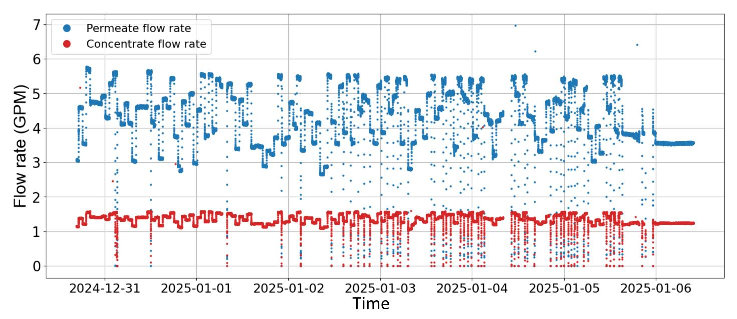
Non-stop 7-day pilot operation. The permeate flow set point was changed remotely and automatically every hour, based on the experimental design.
