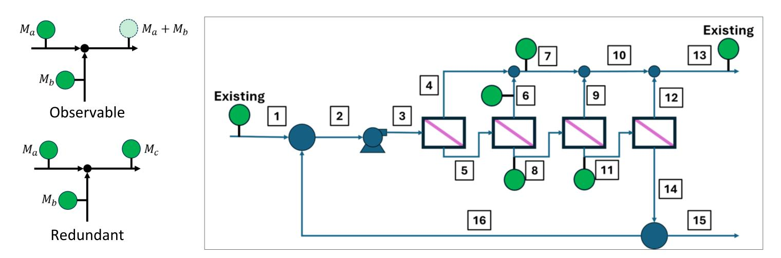
Example of minimum flow sensors needed for full flowrate observability on the pilot
