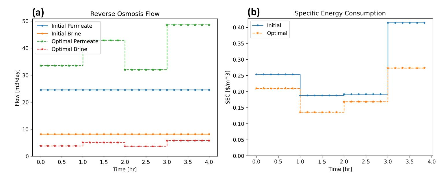
Optimization results for the pilot comparing (a) permeate, brine recirculation, and (b) specific energy consumption cost.
