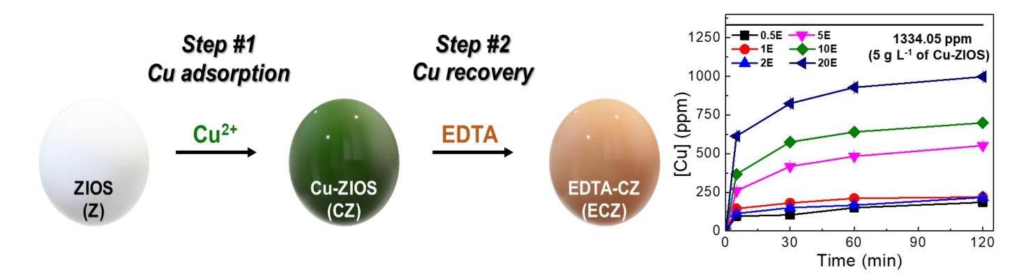
Initial results indicate that Cu metal can be recovered directly from Cu-adsorbed ZIOS (CZ) by a simple EDTA treatment. This has significant potential as an efficient and effective pathway for valorization of Cu from MIW. This approach to Cu recovery adds another potential option for operators to recover Cu from MIW.
