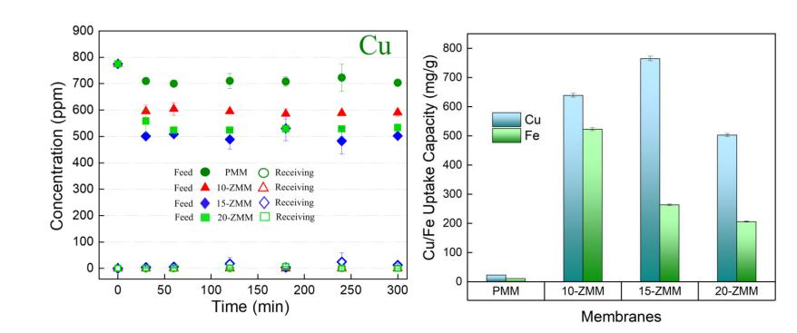
High Cu selectivity behavior of ZMMs after 5 h of exposure in real AMD in diffusion cell. Uptake of Cu and Fe occurs very quickly, with significantly more Cu removal demonstrated by the ZMM membranes compared to pristine PES membrane (PMM)
