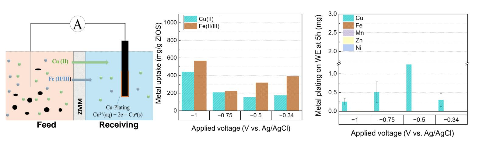
Electrodialysis tests with ZMM using AMD indicate that Cu metal can be selectively recovered by electroplating on a working electrode (WE). Major contaminant is iron. Copper is found in the ZMM and on the WE, with the proportion of Cu recovered on the WE influenced by the applied potential. Demonstrates potential for efficient, selective recovery of Cu metal directly from AMD in a scalable process.
