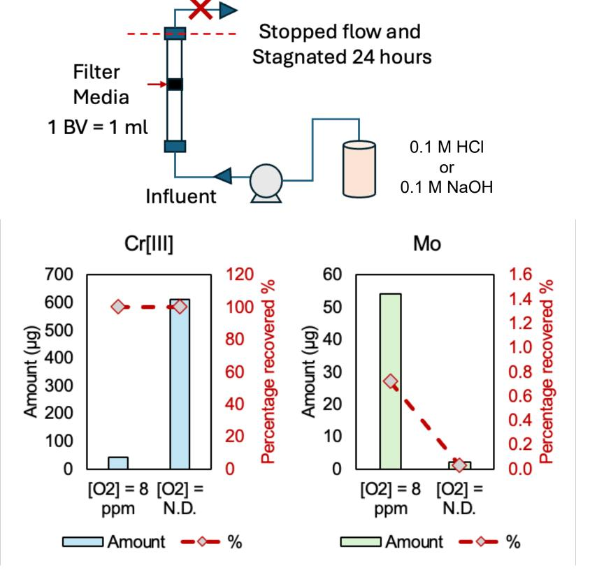
MoS<sub>2</sub> is preserved when treated with acid but undergoes oxidative dissolution in NaOH.
