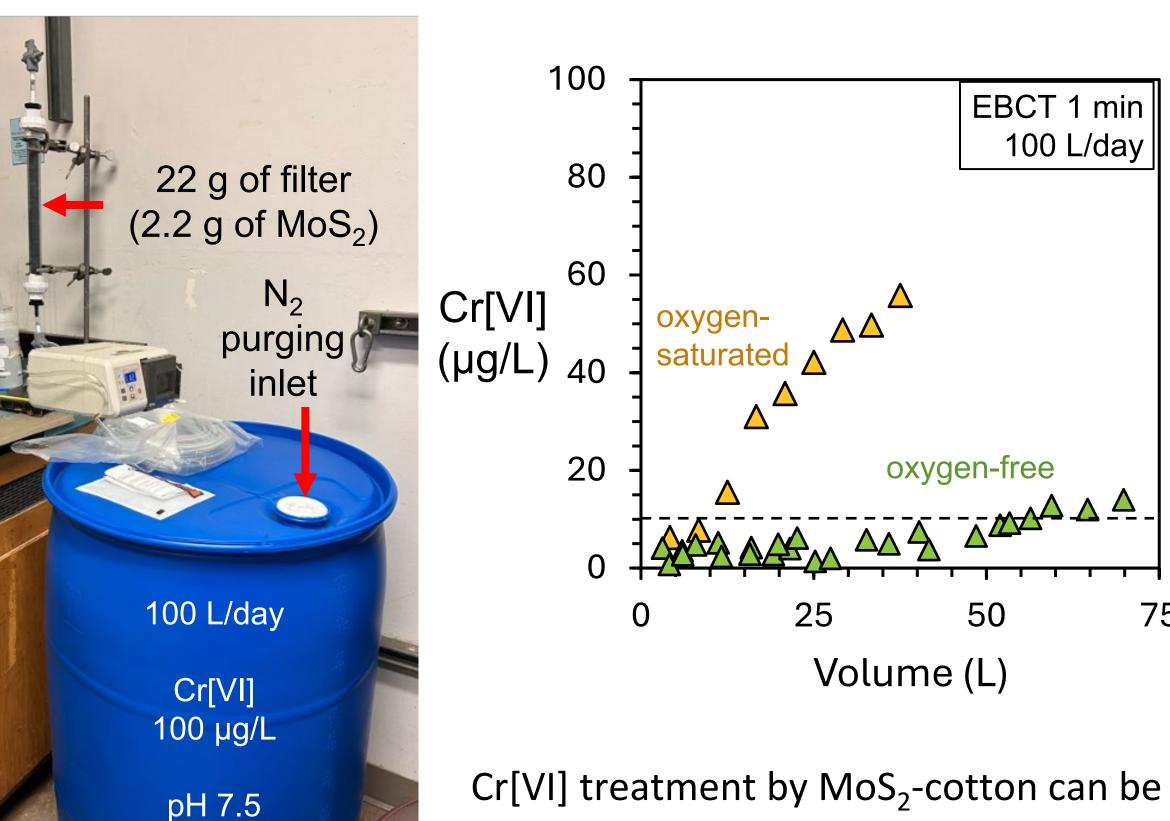
Cr[VI] treatment by MoS<sub>2</sub>-cotton can be effectively at lower empty bed contact time at high pH conditions.
