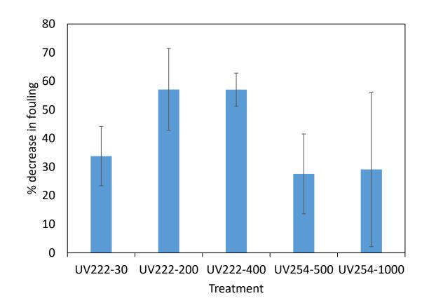
UV222 pretreatment results in 58% fouling reduction, compared to 28-29% fouling reduction from comparable UV254 treatments.
