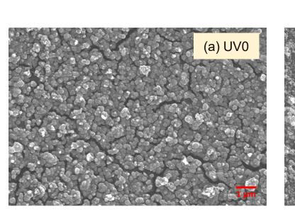
SEM/EDS reveal that UV222 pretreatment results in a less dense fouling layer with more intermixing between organic and inorganic components compared to no UV pretreatment
