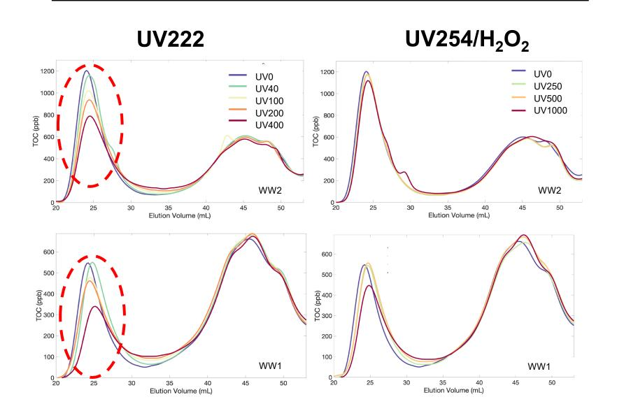
UV222 degrades the large molecular weight fraction in EfOM more than conventional UV254/H<sub>2</sub>O<sub>2</sub>
