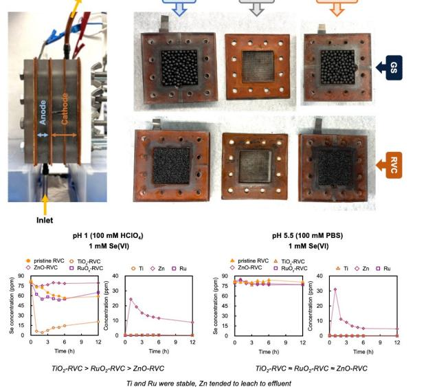
top: 3DER reactor with 3D carbon-based electrode fillers to reduce Se(VI) was investigated; bottom: Evaluation of various catalysts-coated RVC in continuous 3DER showed a better Se(VI) removal by TiO<sub>2</sub>
