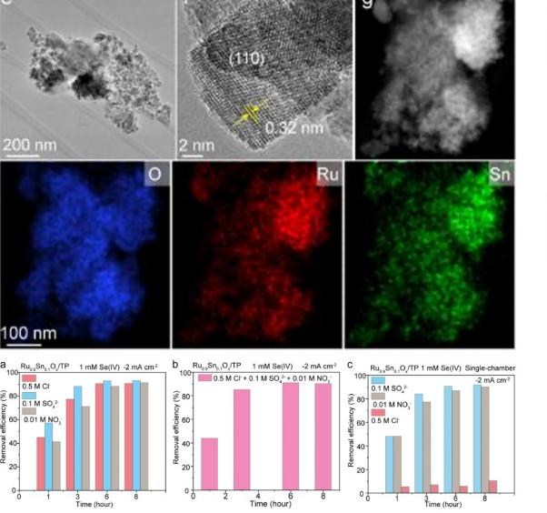
**top**:  $Ru_{0.9}Sn_{0.1}O_x$  supported on Titanium plate SEM and TEM characterizations; bottom: In simulated wastewater containing 1 mM Se(IV) along with competitive anions (0.5 M Cl<sup>-</sup>, 0.1 M  $SO_4^{2-}$ , 0.01 M  $NO_3^{-}$ )
