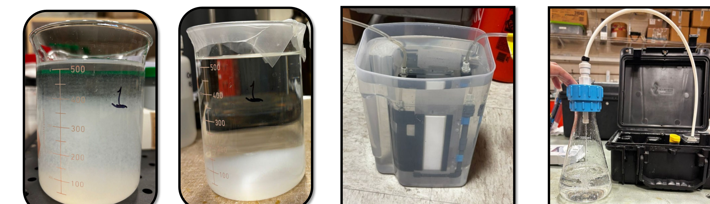
Time = 0 mins Time = 5 mins Cerafiltec filtration SDI measurement Hydrotalcite in-situ formation
