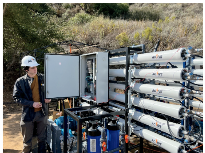
Figure 2: Side-by-side RO trains allowed for a direct comparison of the active membrane technology versus conventional RO.
