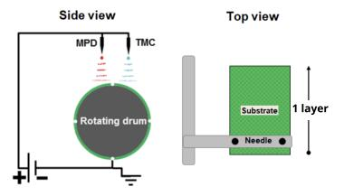
**Figure 1.** Illustration of the lab-scale electrospray process with a single drum. Monomers are deposited by a needle, sequentially, onto a substrate that is attached to the rotating drum where they react to form aromatic polyamide. The lab-scale system can make up to 1 square foot of material and is representative of a continuous process and can be expanded.
