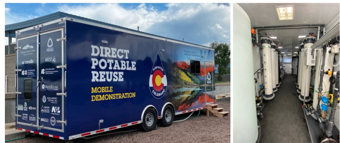
Figure 1. Outside and inside views of the DPR mobile demonstration lab. The six unit-processes installed in the trailer include: ozonation, biologically active filtration (BAF), ultra-filtration (UF), granulated activated carbon adsorption (GAC), ultraviolet irradiation with advanced oxidation (UV-AOP), and chlorination.
