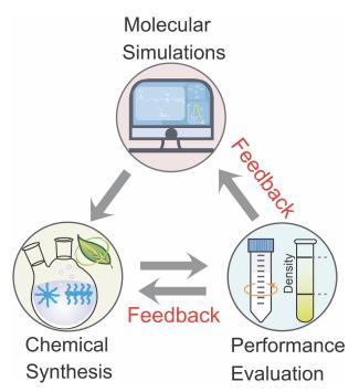
**Figure 1.** Overview of research strategy: molecular simulations to identify functional groups and molecular structures of antiscalants, chemical synthesis of the antiscalants informed by the molecular design principles, and systematic bench-scale performance testing of the synthesized antiscalants.
